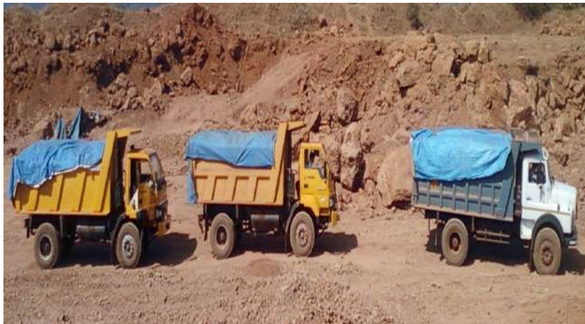
Covering of truck to reduce fly dust while transporting final products on roads
